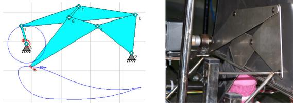
Figure 1. A six-bar linkage. Figure 2. Mechanical construction.
