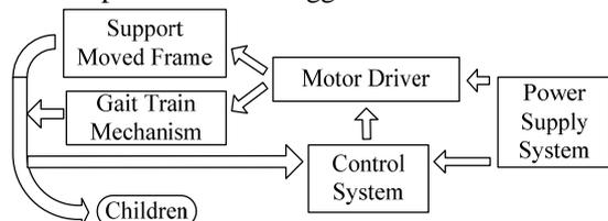
Figure 1 The structure of gait trainer.
