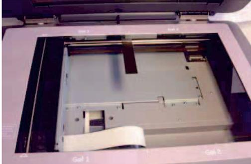
Fig 1. Placing step tablet on the glass plate with the glossy side down.
